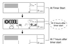
Display shows the timer's ON setting (hours remaining to ON).
