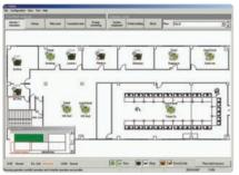
AutoCAD drawing may be imported to TG2000 to display floor screens.
