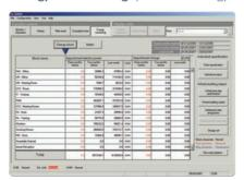
TG2000 in conjunction with energy meters can monitor the energy consumption for each outdoor unit, indoor unit or area. The indoor unit run hours can also be displayed.
