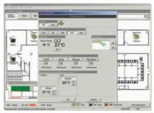
Click on any icons in the floor view to access the remote controller settings. Buttons on the local controllers may be locked (On/Off, Mode, Setpoint, Filter reset).
